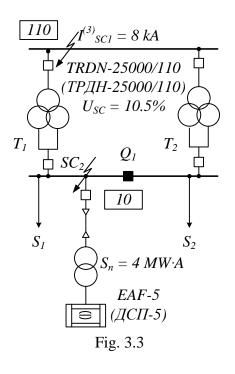
A new electric arc furnace DSP-5 is connected to the main step-down substation 10 kV buses (fig. 3.3).
