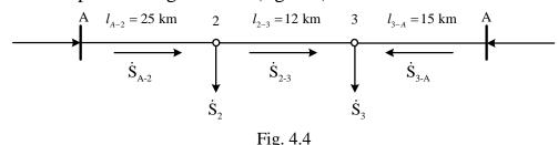
We define the power flow in the ring network using lines length because cables cross-section are the same:
