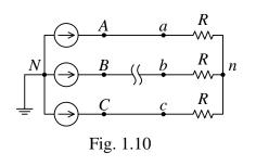
In case of a wire break in phase B the magnitude of the phase voltage of the transformer secondary winding will not change. Basing on this fact we form the equivalent circuit of the transformer secondary winding (fig. 1.10).
