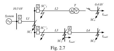
Microprocessor-based inverse time phase protections are installed on 10 kV lines. Inverse time characteristics are determined by the equation:
