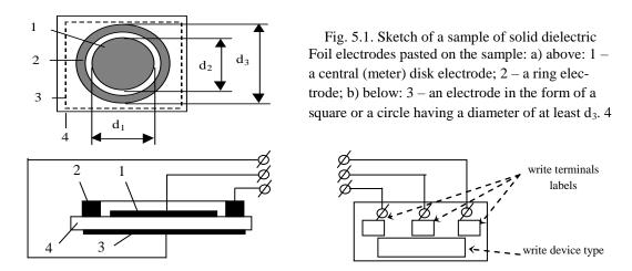
Fig. 5.2. Diagram of dielectric cubic resistance measurement: 1, 2, 3 – electrodes; 4 – dielectric
