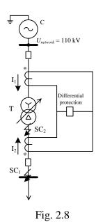
A restrained differential current protection is installed on a transformer (fig. 2.8). The operating characteristic is shown in fig.2.9.
