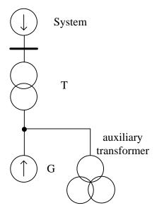
Select the conductive part between the generator and the main transformer of the unit. The unit diagram is shown in fig. 6.8.
