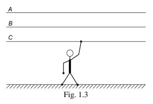
A person touched one wire of a three-phase transmission line rated at 10 kV and 50 Hz (fig. 1.3). The person's resistance is  $R_{man} = 1000$  Ohm, the self-capacitance of each phase with respect to ground is  $C_{11} = C_{22} = C_{33} = 0.256 \,\mu\text{F}$ , and the mutual capacitance between phases is  $C_{12} = C_{13} = C_{23} = 0.115 \,\mu\text{F}$ .
