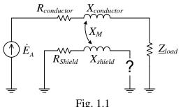
Figure 1.1 shows the single-phase equivalent circuit of a 220 kV three-phase cable line connected to a load with the following impedance:  $\underline{Z}_{load} = 96.61 + j51.21$  Ohm. The cable core conductor and shield have the following parameters:  $R_{conductor} = 5$  Ohm;  $R_{shield} = 20$  Ohm;  $X_{conductor} = 25$  Ohm;  $X_{shield} = 20$  Ohm. The mutual inductance between the core conductor and the shield is  $X_M = 2.5$  Ohm.
