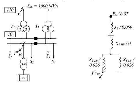
The parameters of the equivalent circuit are  $U_{base} = 10.5 \text{ kV}$
