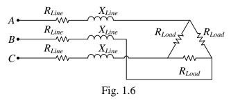
A symmetrical load is connected to a symmetrical threephase circuit with the line voltage  $U_{Line}=380$  V and impedances of  $R_{Line}=X_{Line}=10$  Ohm (fig. 1.6). Determine the value of the
