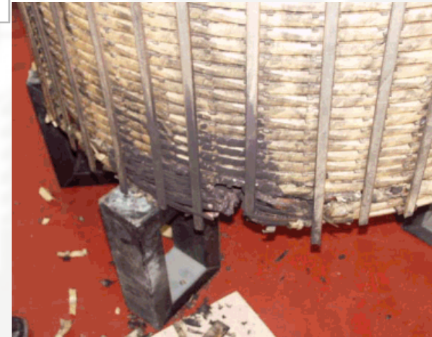
Turn-to-turn short circuit in the transformer
