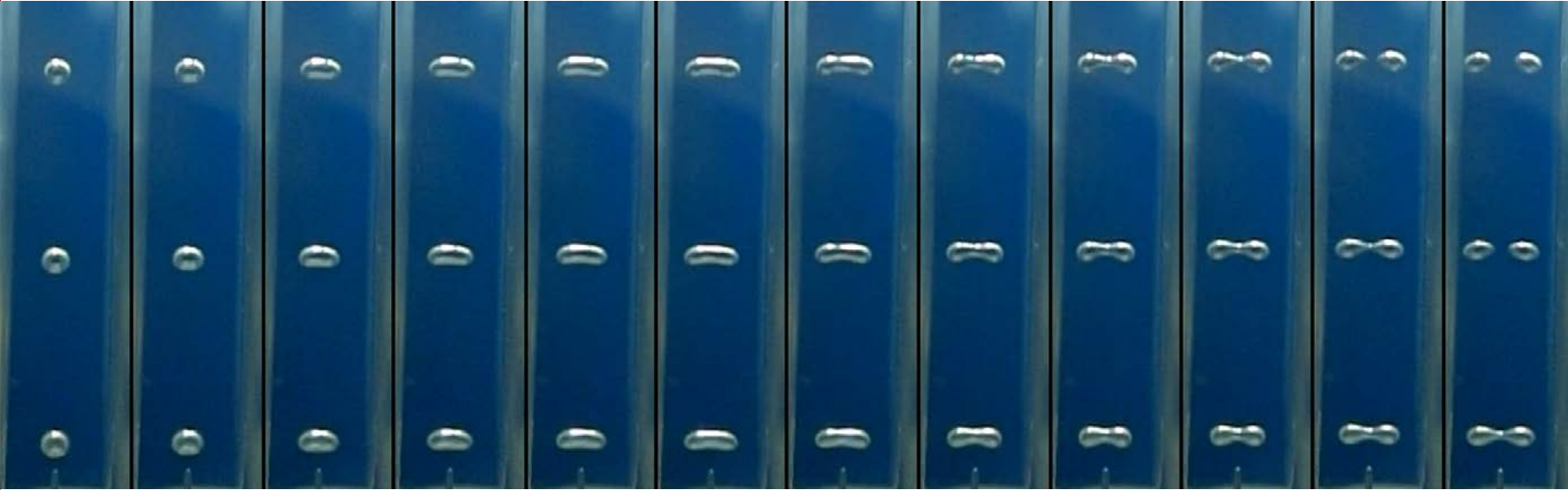
Fig. 9 – PD development in all bubbles simultaneously. PD occurs on the second frame
