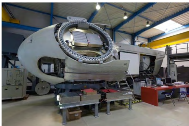
Figure 2 A typical wind turbine drive train
