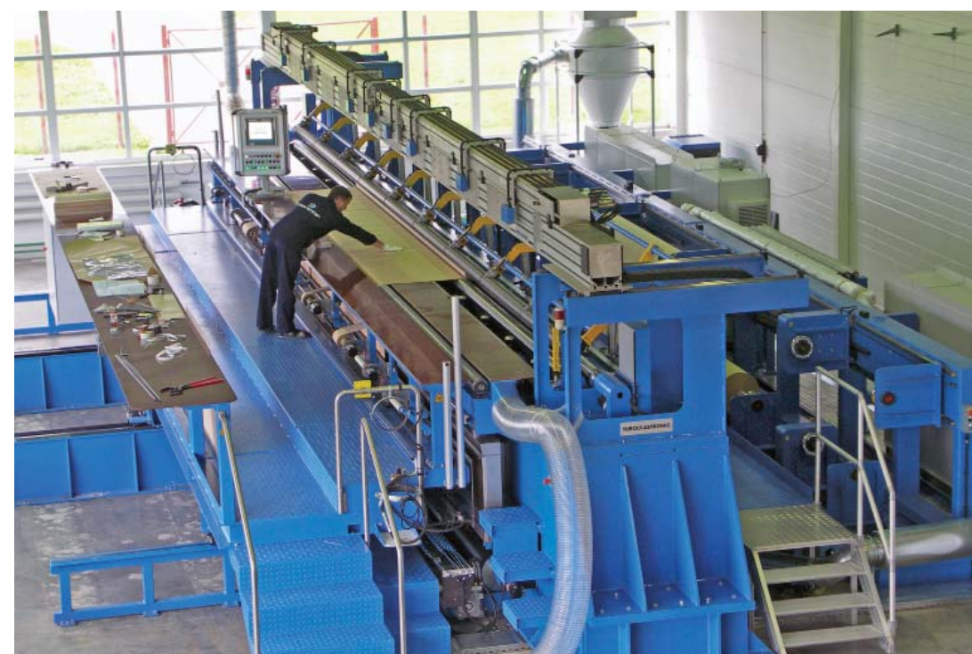
Fig. 1 High-production insulation winding machine 252–1200 kV
